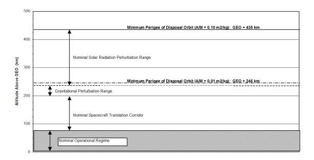
Figure 4.6-1: IADC Rationale for GEO minimum perigee equation
