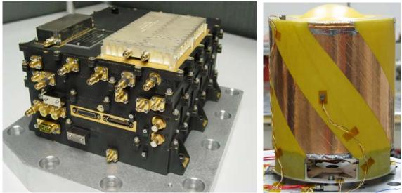
Figure 1: Electra UHF Transceiver and UHF Antenna
