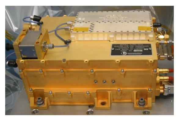
Figure 1: Electra-Lite UHF Transceiver
