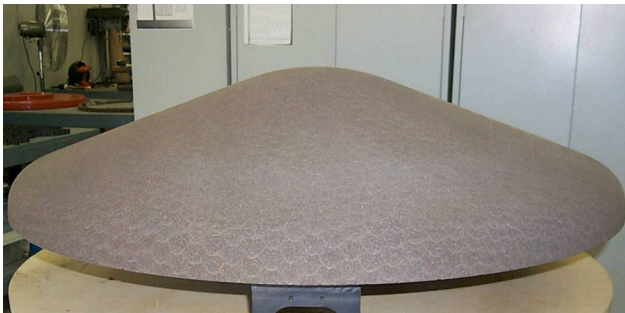
Figure 4. One meter ablative aeroshell with ARA's PhenCarb 20 TPS material.
