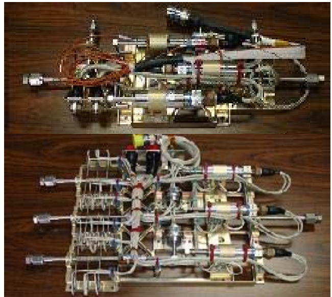
Figure 4. NEXT EM High Pressure Assembly (top) and Low Pressure Assembly (bottom) from the Propellant Management System
