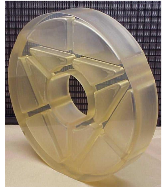
Shaped Zerodur Primary Getting Fiducials
