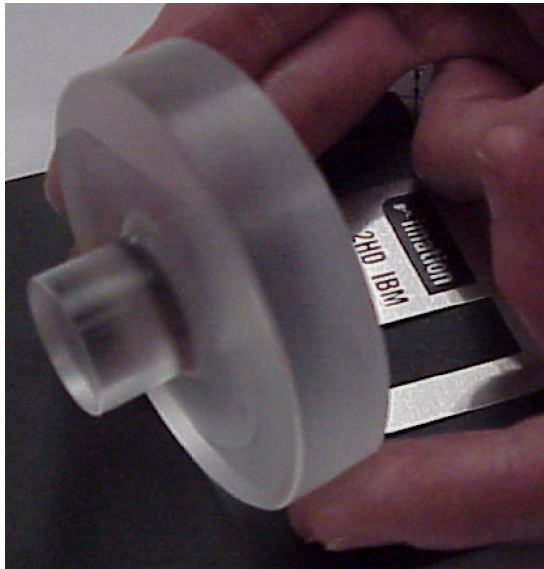
Fused Silica Secondary Proof Article
