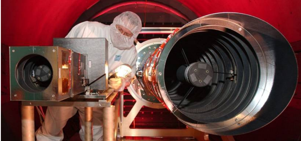
Figure 3. The MRI (left) and HRI (right) telescopes are prepared for low temperature testing. These tests were used to determine the adjustments needed to set the focus of the instruments at the cold operating temperature.
