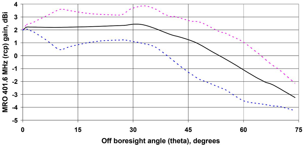
Figure 5.2-3 MRO 401.585625 MHz (RCP) gain pattern
