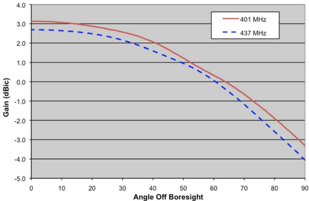
**Fig. 6.2-1: MAVEN UHF Antenna Gain Pattern**
