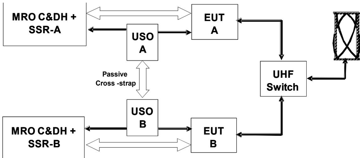
Figure 5.2-1 MRO/Electra UHF subsystem block diagram and interfaces with C&DH and SSR
