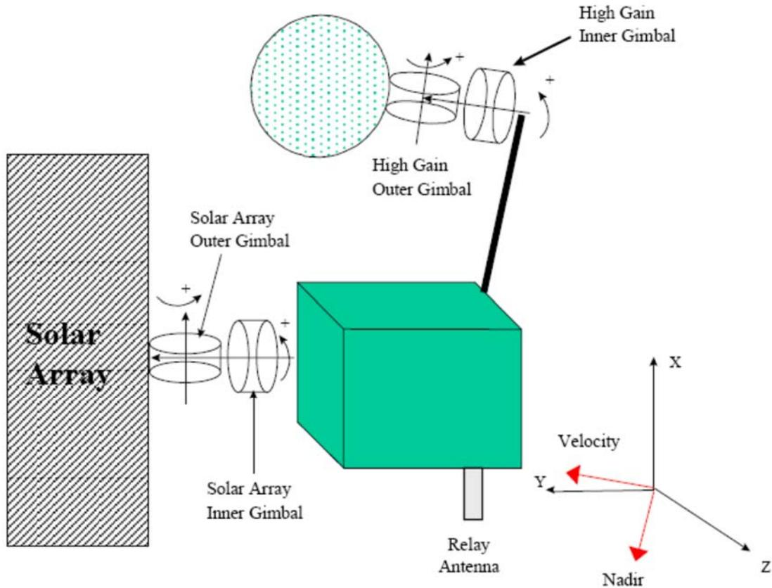
Figure 4.4-1 Odyssey and UHF antenna geometry
