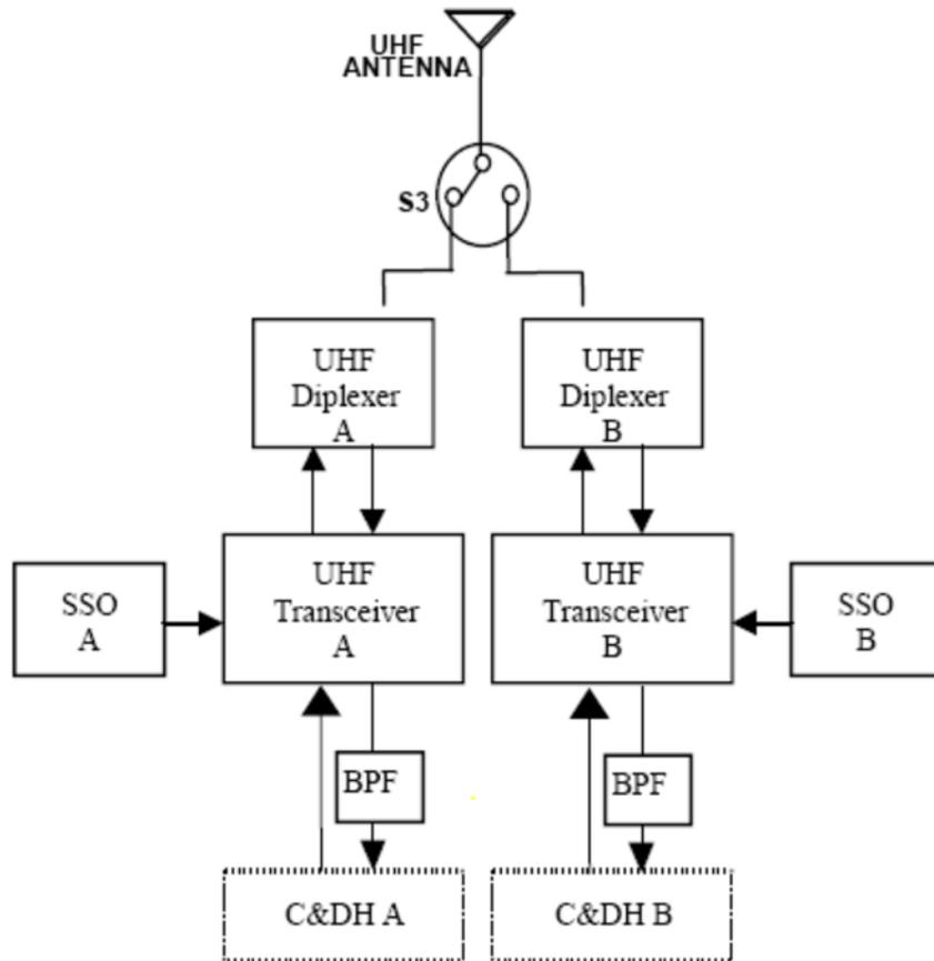
**Figure 4.2-1** Block diagram of Odyssey UHF subsystem
