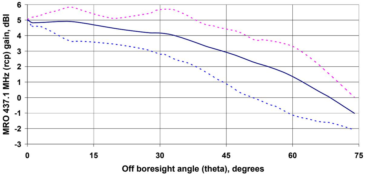
Figure 5.2-2 MRO 437.1 MHz (RCP) gain pattern
