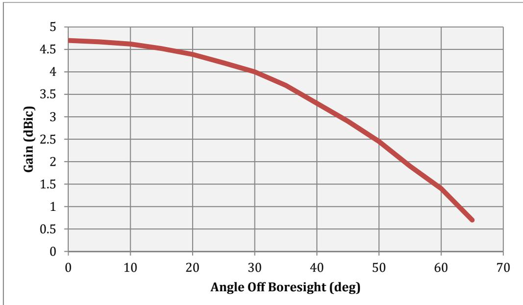
**Figure 7.2-1: Preliminary ExoMars/TGO UHF Antenna Gain Pattern**
