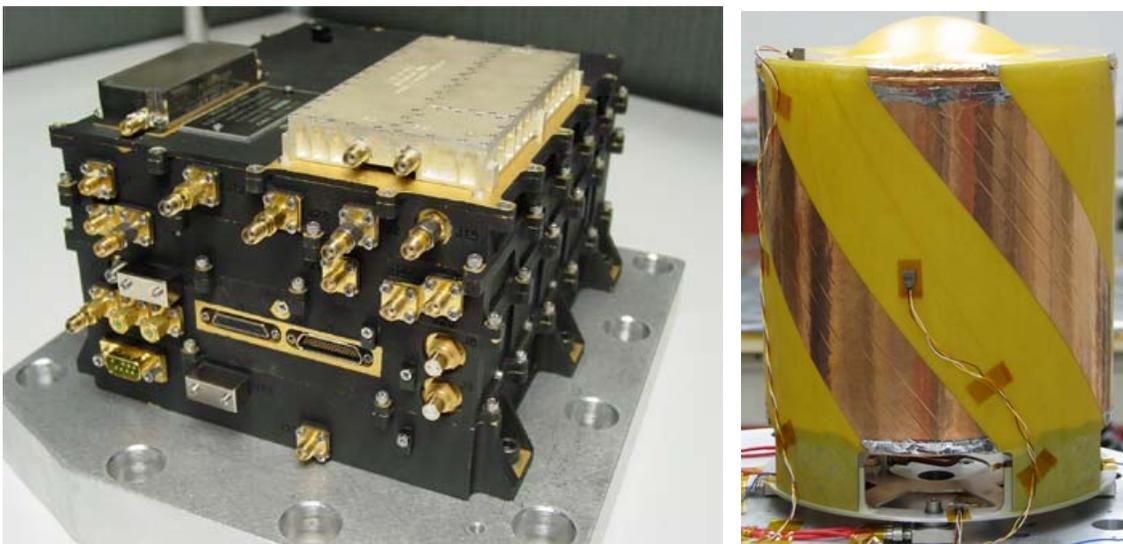
*Figure 1: Electra UHF Transceiver and UHF Antenna*
