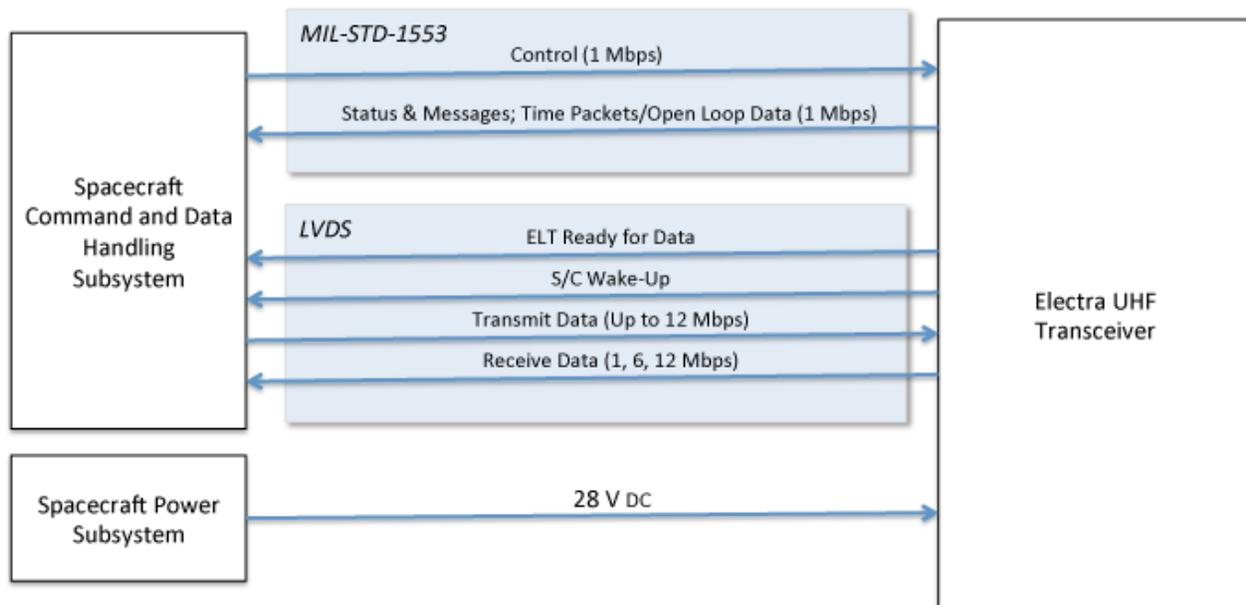
**Figure 2: Electra Lite – Spacecraft Bus Interfaces**
