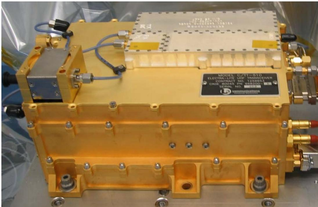
**Figure 1: Electra-Lite UHF Transceiver**
